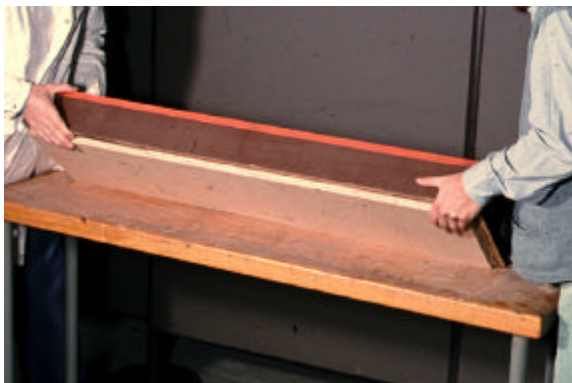
20. After hardening, the box is turned over
