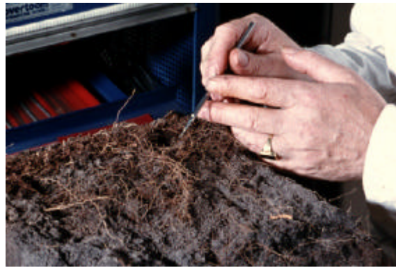
23. Loose material is removed carefully
