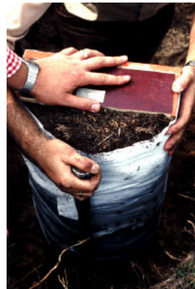
13. The box and soil column are detached from the face and tilted; bandages prevent soil falling out
